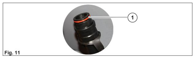
Check the seal at the drain hose daily and replace it after 125 operating hours at the latest.
