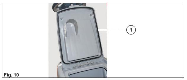
Check the function of the seal in the tank cap daily and replace the seal if damaged.
