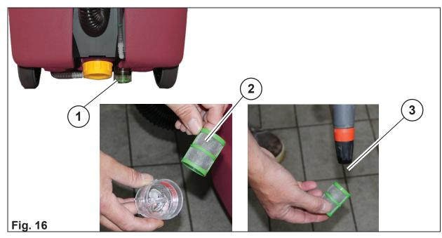
Clean the sieve insert of the fresh water filter weekly. The fresh water filter is located at the rear right beneath the machine **Fig. 16-1**.
