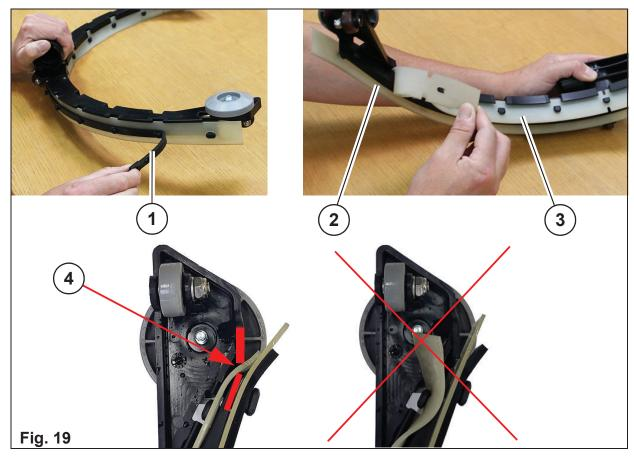
Check the sealing strip and the slot strip at the squeegee weekly for wear and damage. If the edge of the sealing strip is worn or damaged, turn or replace the sealing strip. Each sealing strip can be used four times before it needs replacing.
