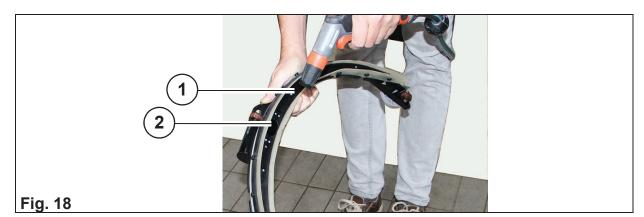
Check the squeegee **Fig. 18-1** and the suction channel **Fig. 18-2** daily for soiling and foreign particles and clean them as required.
